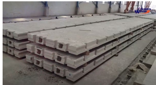
Gambar 4. Panel beton SpRigWP.
