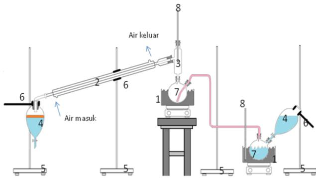
Gambar 1. Skema Alat Metode *Steam Distillation*
