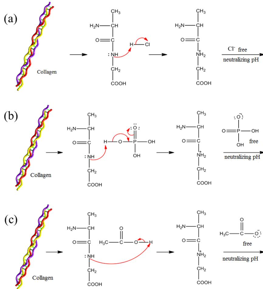
Figure 4. Proposed reaction mechanism in the acid pre-treatment process
