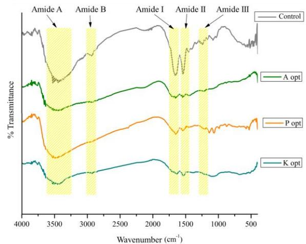
Figure 9. FT-IR spectra of gelatin using acid pre-treatment
