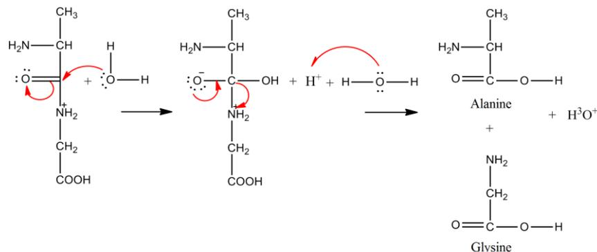
Figure 5. Proposed reaction mechanism in the extraction process
