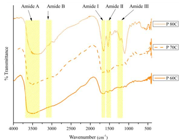
Figure 7. FT-IR spectra of gelatin using P pre-treatment
