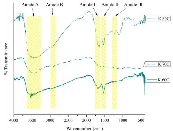
Figure 6. FT-IR spectra of gelatin using K pre-treatment
