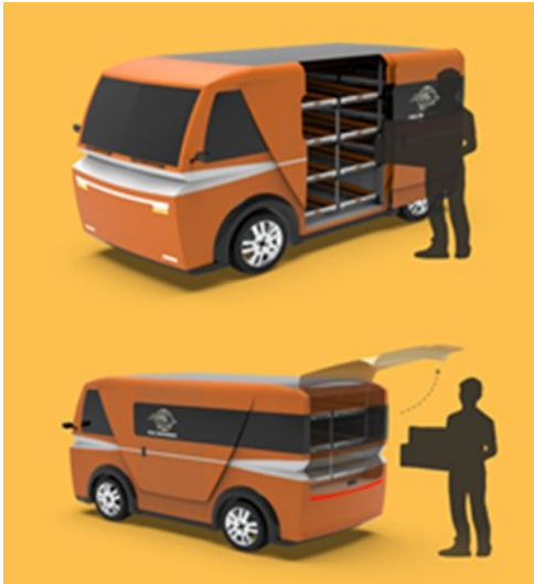
Figure 6. Implementation of gravity flow tube storage system on a delivery vehicle design. There are two storage systems: front and rear storage. Front storage system can be accessed through two side doors of the vehicle (right or left door), while rear storage can only be accessed through the rear door.
