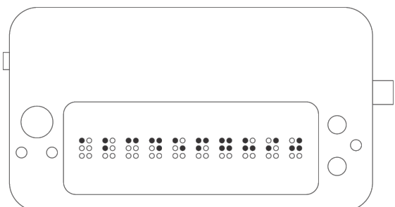
Figure 10. Third layout. The third layout has the power button on the left side of the product. The mode button has the bigger size than the content button. The scroll up and down button is placed on the right in the front side of the product. The audio button is place besides the scroll button. The volume adjuster is placed in the right side of the product.
