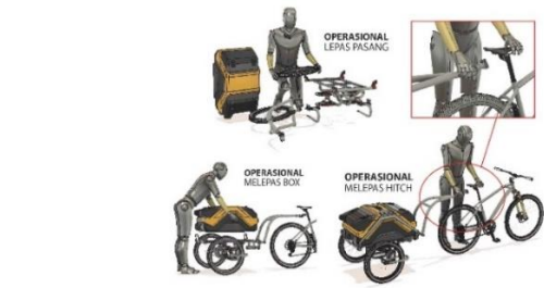
Gambar 4. Operasional lepas pasang komponen bike trailer
