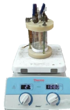
Figure 1. Dead-end mode ultrafiltration Reactor.
