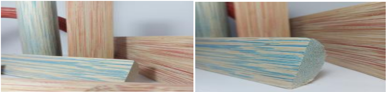
Gambar 11. Hasil eksperimen material rotan resin-infusion.
