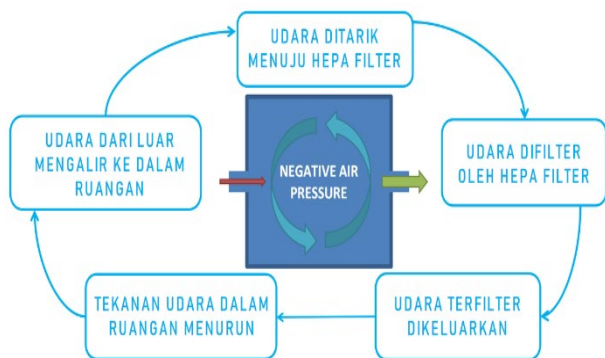
Gambar 4. Skema cara kerja negative pressure isolation system.
