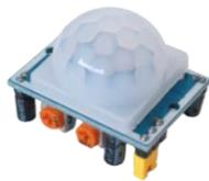
Gambar 4. Sensor Passive Infrared Receiver (PIR).
