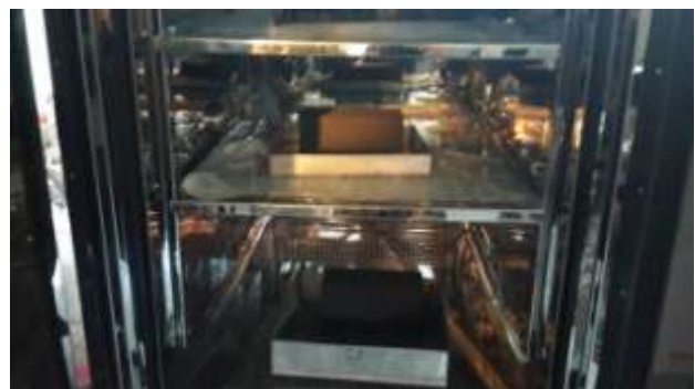
Gambar 4. Proses Steam Curing Paving
