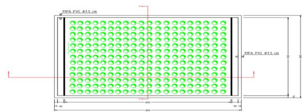
Gambar 11. Denah unit constructed wetland .
