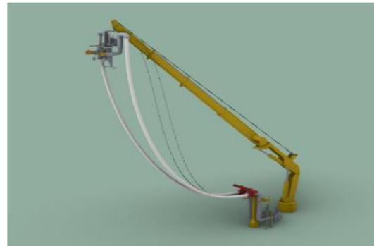
Gambar 10. Desain 3D LNG *knuckle boom*.
