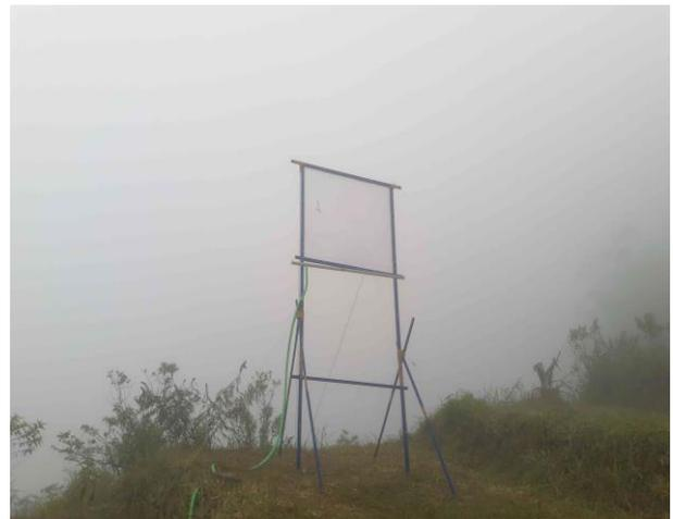
Gambar 1. Fog catcher mesh 1 m x 1 m.
