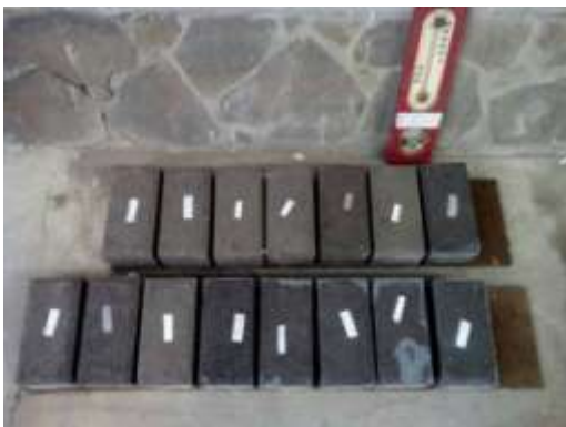
Gambar 1. Curing dan Storage Paving
