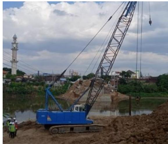
Gambar 2. Crawler Crane Hitachi Sumitomo DC88 SCX500.
