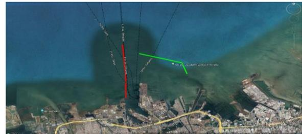
Gambar 5. *Layout 3* pemodelan *floating breakwater*.
