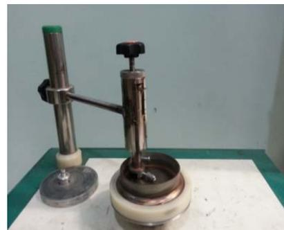
Gambar 2. Tribometer Tipe Pin on Disk
