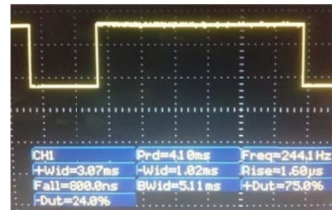
Gambar 10. Duty cycle 75% (Kondisi: freq 244,1 Hz, On Duty cycle 75%, OFF Duty cycle 24%)
