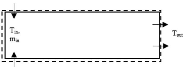
Gambar 5. Control volume perhitungan termodinamika
