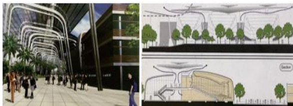
Figure 6. Atrium as a meeting place for users who acts indoor spaces but with an outdoor atmosphere, to manipulate its functions as wind management and also a place for user activities [6].
