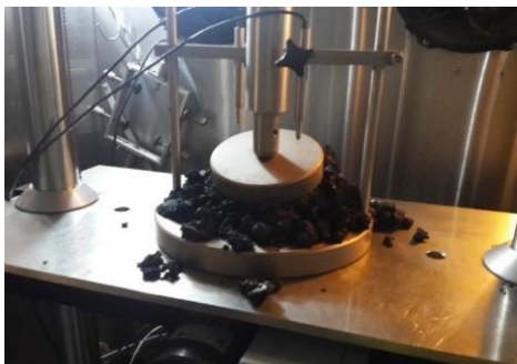
Figure 6. Samples Experiencing Collapse.
