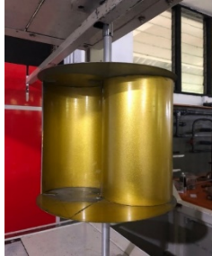
Gambar 2. Turbin Angin Savonius
