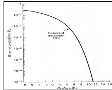
Gambar 1 Probabilitas Bit Error BPSK [1].
