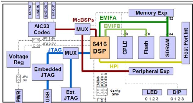
Gambar 2. Blok Diagram TMS320C6416T [2]
