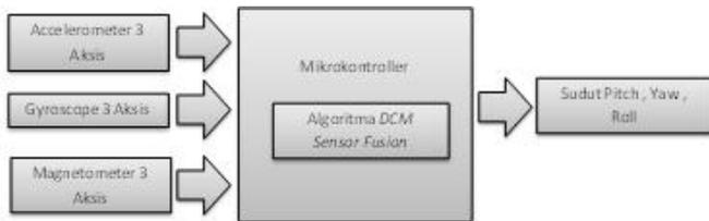
Gambar. 1. Diagram Blok Sistem *Inertial Measurement Unit*.
