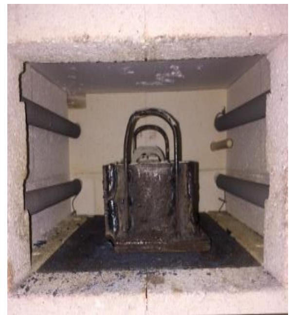
Figure 2. Reaction Pack in the Furnace.
