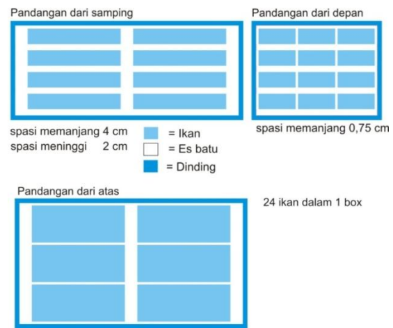
Gambar 4 Hasil Simulasi Cold Storage Konvensional
