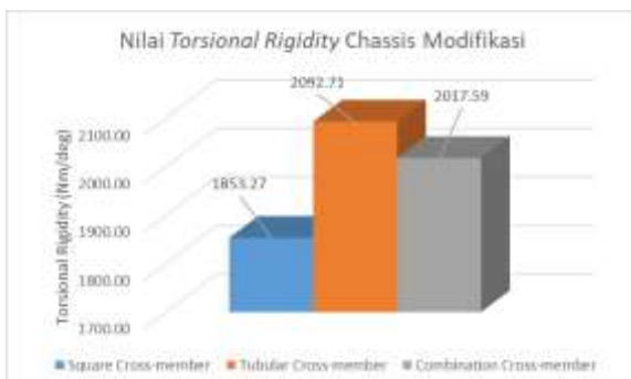
Gambar 9. Grafik perbandingan nilai torsional rigidity antar variasi desain cross-member .
