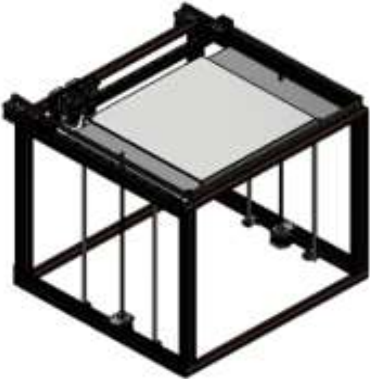
Gambar 2. Isometri mesin 3D printer.
