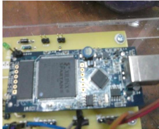
Gambar 2. Board FPGA Spartan 3E
