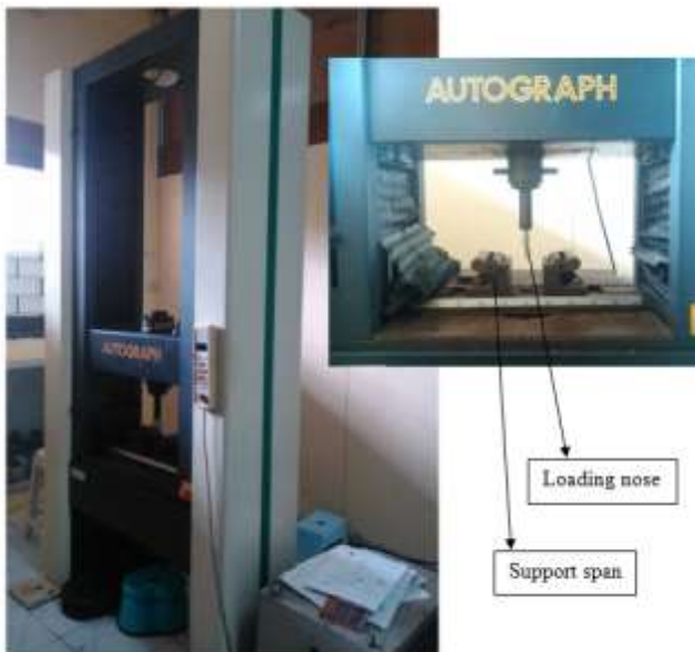
Gambar 13. Mesin uji bending AUTOGRAPH
